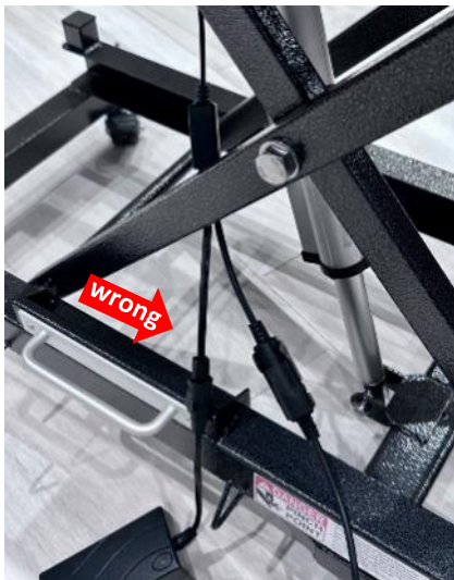
INCORRECT WIRE PLACEMENT: Wires cross over the frame. High risk of wires being pinched and possibly sheared during operation.
