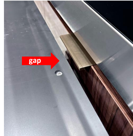
CORRECT POSITION: By leaving a gap between the front of the tabletop and the drawer pull, the tabletop will avoid the drawer pull when rising.
