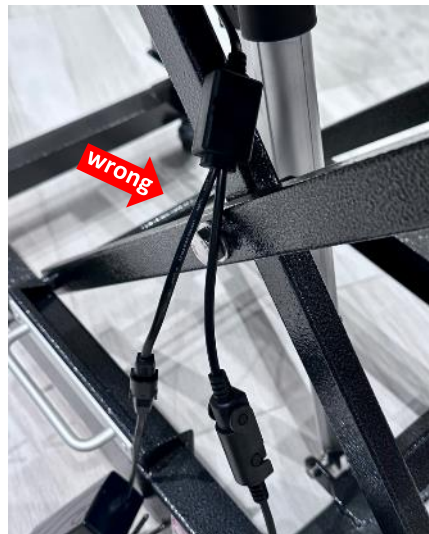
INCORRECT WIRE PLACEMENT: Wires cross over the frame. High risk of wires being pinched and possibly sheared during operation.
