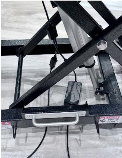
CORRECT WIRE PLACEMENT: Wires completely under the frame. No risk of wires being pinched and possibly sheared during operation.
