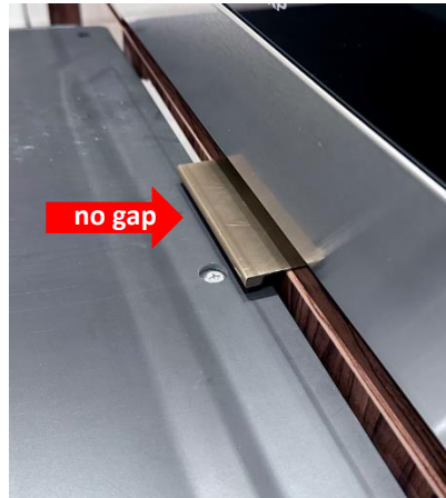
INCORRECT POSITION: Because there is no gap between front of tabletop and drawer pull, the tabletop will run into drawer pull when rising and may cause damage.
