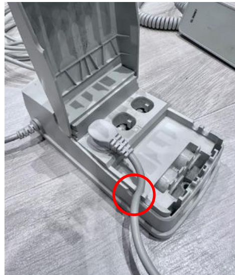
Step 2: Connect the power box so that the wire is secured into the LEFT slot and travels out through the side notch (see red circle over side notch).
