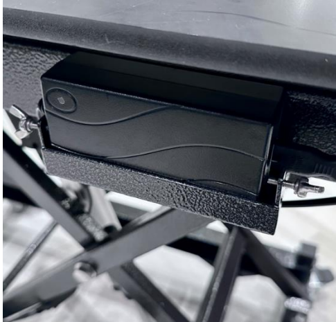
Secure power box in cradle by tightening wing nuts.
