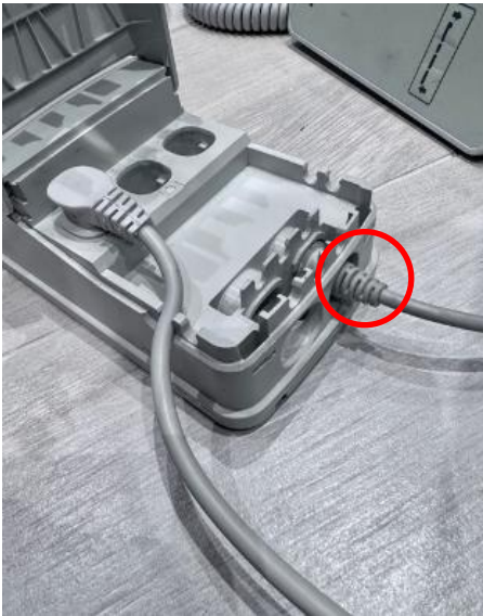
Step 3: Connect the hand controller into the lower right slot by pressing it firmly (see red circle).
