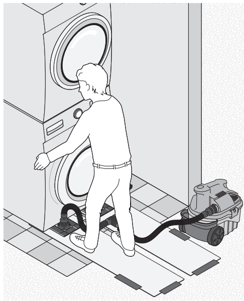
Rough Surface Adapters to create a smooth track
